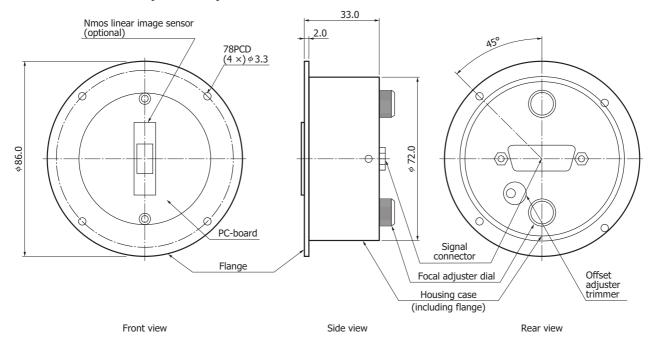
The focal position can be adjusted backward within the range from 0 to 4.5 mm (circuit stroke length) with a focal adjustment dial.
