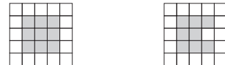
This is defined as defect cluster. This is not defined as defect cluster.
