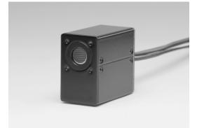
The H10682 series is a photon counting head device consisting of a metal package photomultiplier tube, along with a high speed photon counting circuit and a high-voltage power supply circuit. The high voltage supply for photomultiplier tube and the discrimination level are preset to optimum values, allowing photon counting measurement by just connecting a +5 V supply.
