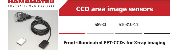
The S8980 is an FFT-CCD image sensor suitable for intra-oral X-ray imaging in dental diagnosis. The S8980 has 1.5 mega (1500  $\times$  1000) pixels, each of which is 20  $\times$  20  $\mu$ m in size. The FOP (fiber optic plate) used as an input window is as thin as 1.5 mm, making high resolution as well as highly resistant to X-ray irradiation. The scintillator coated on the FOP is optimized to have high X-ray sensitivity and high resolution (20 Lp/mm).
