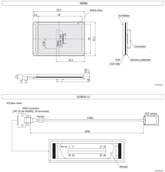
\* The shield of cable and the shroud of MDR connector are short-circuited. Take due care of EMC and ESD when connected to 0 V reference and the ground.
