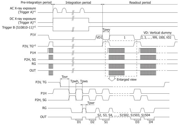
\*1: Trigger A (S8980) is the same as AC/DC X-ray exposure form.
