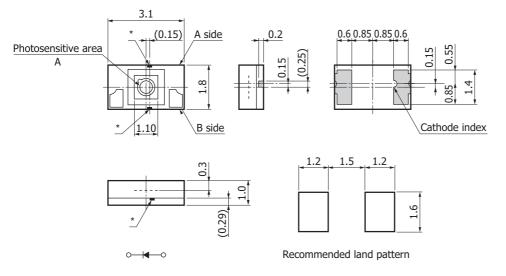
Tolerance unless otherwise noted:  $\pm 0.2$ Photosensitive area position accuracy: X, Y $\leq \pm 0.3$ Values in parentheses indicate reference value. \* Package side
