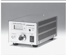
By adjusting the current flowing through the thermoelectric cooler in a one-stage or twostage thermoelectrically cooled detector, the C1103-04 maintains the detector element at a constant temperature. The cooling temperature can be easily set by using the control knob on the front panel.
