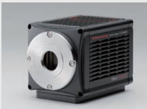
▲ ORCA-Flash4.0 V3 Digital CMOS camera C13440-20CU
