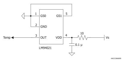
Note: For the analog temperature sensor, use the LM94021 by Texas Instruments. Connect pins 1 and 5 of the analog temperature sensor to ground.
