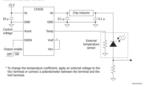
Note: For the analog temperature sensor, use an LP731JTTE102F3600 by KOA.
