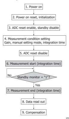
Sensitivity variation can be decreased using the compensation coefficient which is calculated from the integration time measurement result. Explanation of compensation method is shown as follows.
