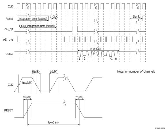
Parameter Symbol Min. Тур. Max. Unit Clock pulse frequency 0.1 2 MHz fop 1 Clock pulse width tpw(clk) 150 5000 \_ ns Clock pulse rise/fall times 0 20 tr(clk), tf(clk) 30 ns High 2 --Reset pulse width clocks tpw(res) Low Number of pixels + 16 \_ \_ Reset pulse rise/fall times tr(res), tf(res) 20 30 0 ns
