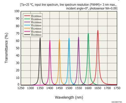
• There is tolerance in filter control voltage for arbitrary peak transmission wavelength from unit to unit. The individual data for V\(\lambda\)1650nm and V\(\lambda\)1350nm at Ta=25 °C is to be described in an inspection sheet attached with a product on delivery.
