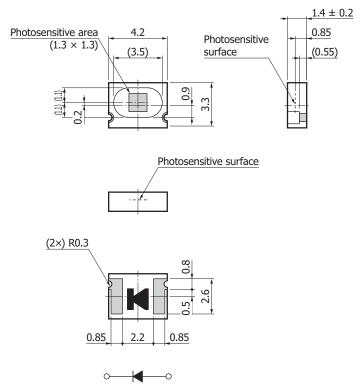
Tolerance unless otherwise noted:  $\pm 0.15$ ,  $\pm 2^{\circ}$ Chip position accuracy: with respect to package center X $\leq \pm 0.2$ , Y $\leq \pm 0.2$ ,  $\theta \leq \pm 2^{\circ}$
