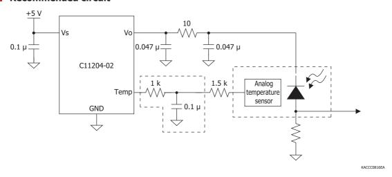
Note: For the bypass capacitor to connect to Vo, use a high-withstand-voltage, low-ESR capacitor. Provide a noise filter near the Temp pin.
