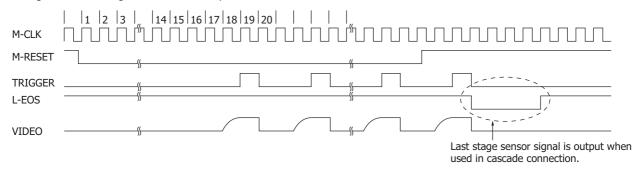
Timing chart of second and subsequent stage sensors when used in cascade connection
