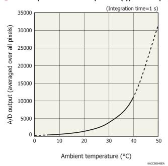
$\mbox{\ensuremath{\mathsf{A}}/D}$  output is the sum of the sensor and circuit offset outputs and the sensor dark output.
