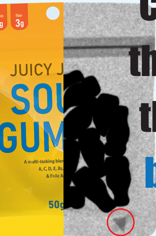
▲ Package seal inspection (Left: Visible image, Right: X-ray image)
