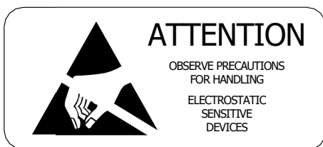
[Figure 4] Electrostatic warning label example
