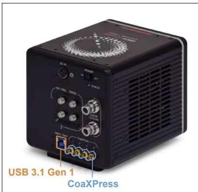
Fig. 3-2. CoaXpress and USB 3.1 Gen 1
