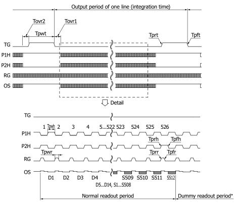
\* It is necessary to wipe out the dark current generated in the horizontal shift register when integration time is set longer than normal readout time.
