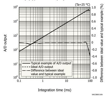
A/D output is the output with dark output subtracted when light is input. The difference between the ideal value and typical example contains a measurement error. The smaller the A/D output, the larger the measurement error
