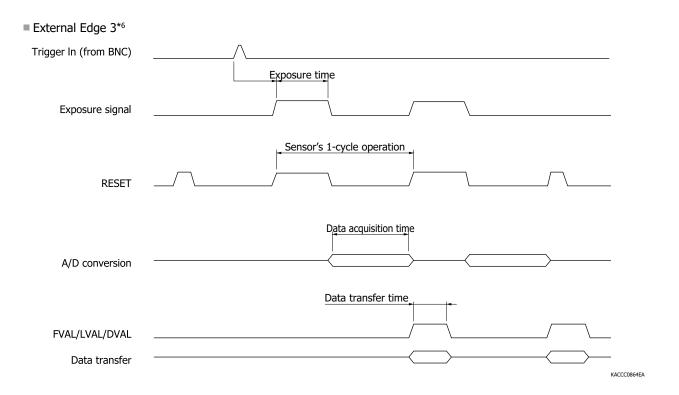
\*6: Data of multiple lines can be acquired with a single external trigger signal as wall as similar operation to External Edge 1.
